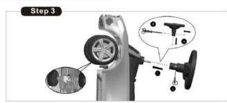
3. Hold the J-shaped stick at the bottom, then place the steering wheel over the J-shaped stick, insert the bolt and tighten the nut with a screwdriver(not included).
